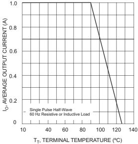
Fig. 1 Forward Current Derating Curve
